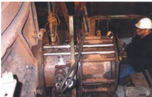
A specially designed orbital milling device machines the trunion to 510mm diameter prior to finish turning down to 500mm diameter to accept an EN14a shrink-fitted ring.
