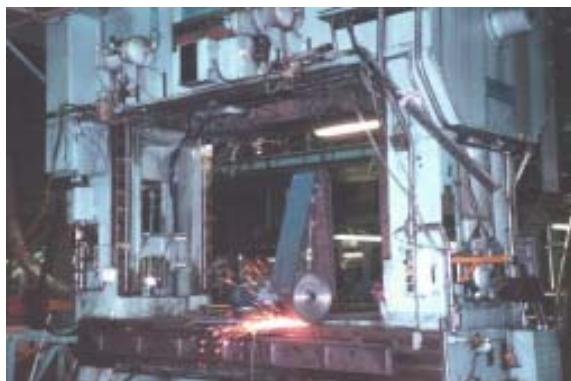
Metallock's insitu grinding machine for metal can conversion presses, used to press ring pulls, restores the overall flatness and paralellism with the upper ram to within 0.04mm TIR on a lower bed die of 1270mm by 760mm.
