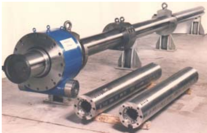
Metallock's new modular boring bar can be extended from 2 metres to 12 metres long and is capable of machining up to 5 metres diameter.
