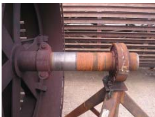
The worn journal, before being orbitally machined, thermally sprayed and then finish turned to accept a new bearing sleeve.
